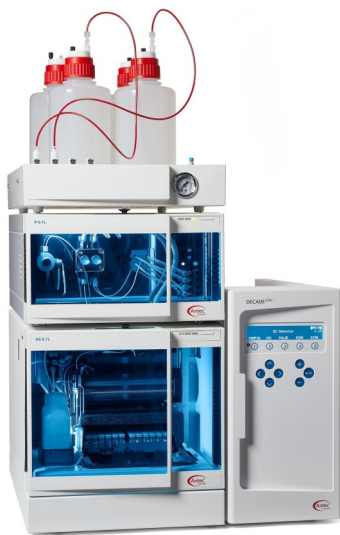
Figure 1. ALEXYS Carbohydrate Analyzer— isocratic, consisting of the ET 210 eluent tray (for N 2 blanketing), a P 6.1L pump with solvent selection valve and dual channel degasser, AS 6.1L autosampler and DECADE Elite electrochemical detector.
